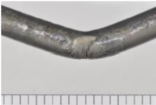
Figure 11. Crack on Exterior of Thermocouple Sheath
