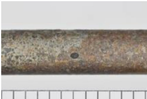
Figure 9. Pit on Exterior of Thermocouple Sheath
