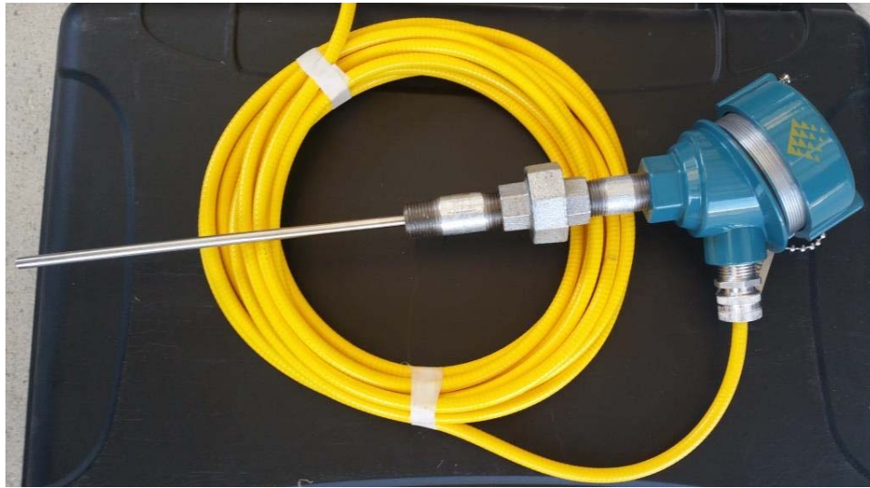
Figure 9. Daily Model 310 Industrial Sensor Used in the Transient Temperature Tests
