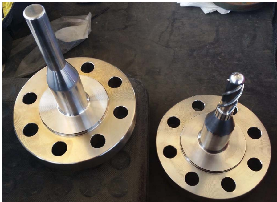
Figure 2. Thermowells Used in the Temperature Transient Tests
