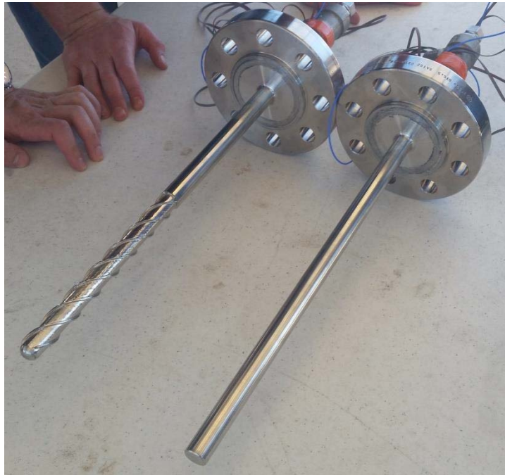
Figure 3. Thermowells Used in the Vibration Tests in the 12-Inch Test Run
