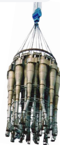
FIGURE 1: FCC Cyclones & Cyclone Exit Legs
